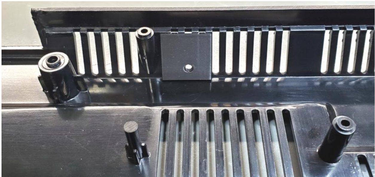
Figure 11a: LED mounting bracket placement in lower case housing
